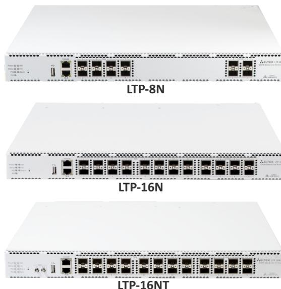
Station equipment (OLT) is designed to provide broadband access over Passive Optical Network (PON).
